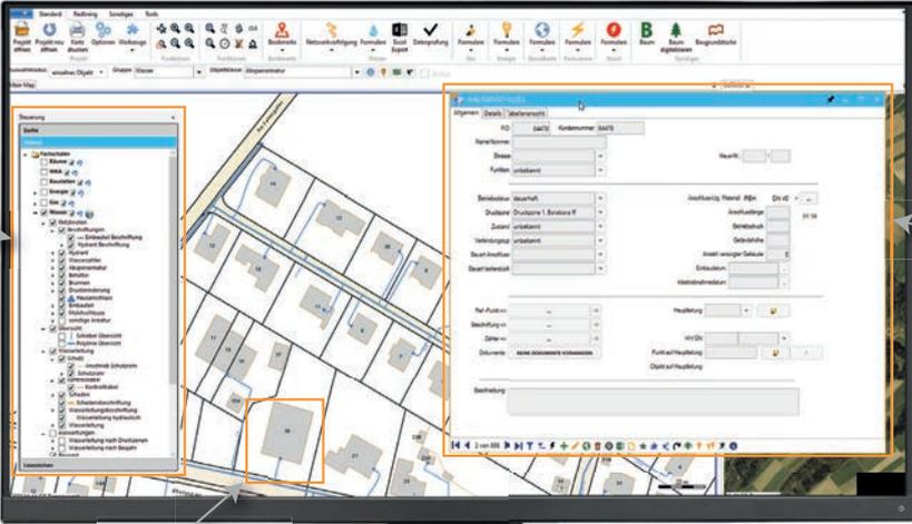
The screenshot shows the MapEdit desktop application. The main window displays a map of a water network with various pipes and structures. On the left, there is a 'Layer' panel with a tree view of data layers. On the right, there is a 'Properties' window for a selected object, showing fields for name, ID, and various technical specifications. Three callout boxes provide additional information:
