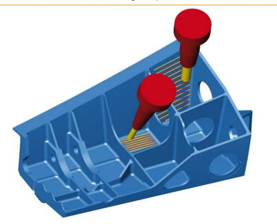
**Project**: Flat surface milling 10x faster by using special conical cutters with slightly convex curvature. Milling time for this lightweight aerospace part:
