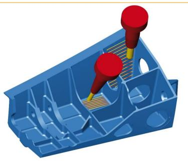
**Project**: Flat surface milling 10x faster by using special conical cutters with slightly convex curvature. Milling time for this lightweight aerospace part: Total 2h05min instead of 10h30min
