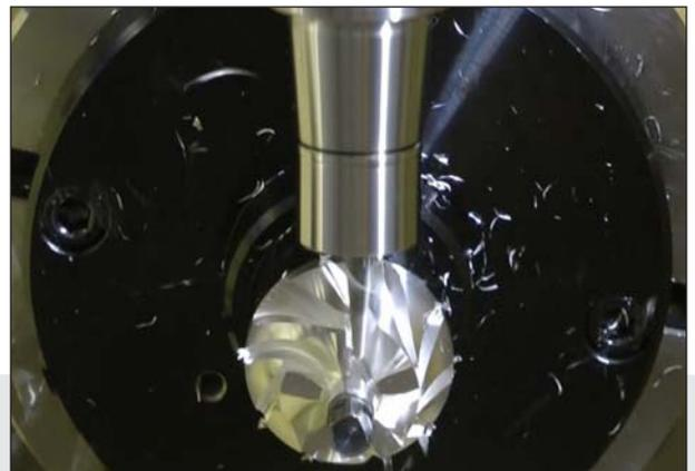
A variety of innovative applications for specific products like tyre molds, turbine blades and impellers enable and simplify the programming of complex handling, lower the machining time and improve finished quality.
